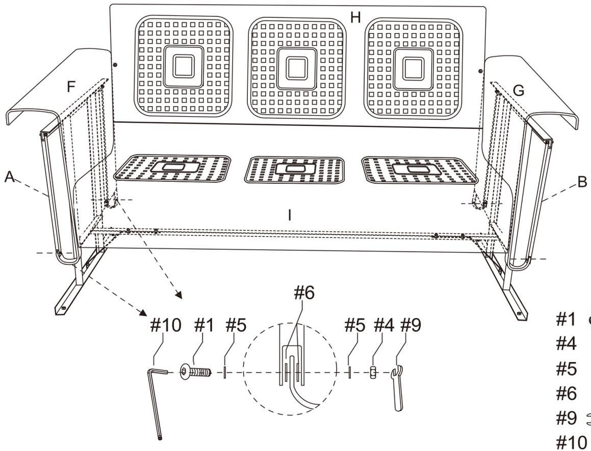
Step 7. Attach connecting wire (part E) to arms (parts F & G) using metal washers (part #5), self-locking nuts (part #4) and wrench (part #9).
