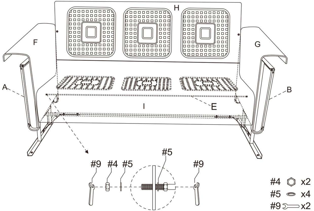
Step 8. Attach connecting wire (part E) to arms (parts F & G) using metal washers (part #5), self-locking nuts (part #4) and wrench (part #9).
